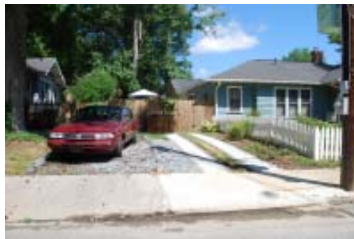
Off-street parking is very limited in some parts of the historic districts. In this case the Historic Preservation Commission granted a COA for a driveway constructed of parallel concrete runners so that the homeowner could have off-street parking with as little impact to the character of the neighborhood as possible.
