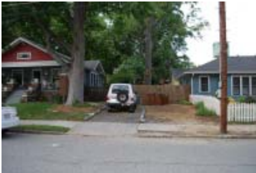
Off-street parking is very limited in some parts of the historic districts. In this case the Historic Preservation Commission granted a COA for a driveway constructed of parallel concrete runners so that the homeowner could have off-street parking with as little impact to the character of the neighborhood as possible.
